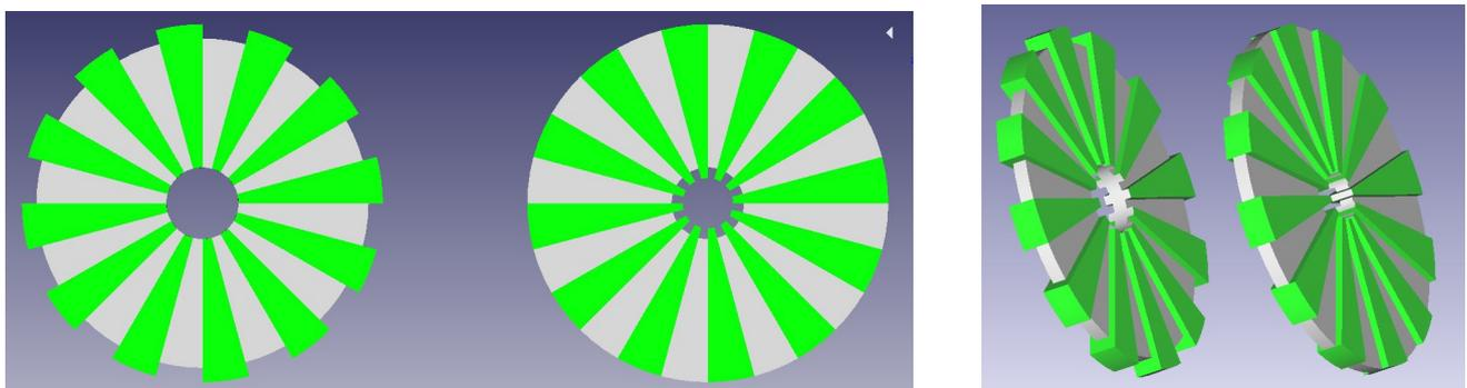
The “stack” comprises two alternating disk designs that have matching raised segments and are made of a conducting material. In this example each segment is 15 degrees wide with 15 degree gaps. But so long as the gaps are no wider than the raised segments other angles can be used. One disc type has the segments projected outside the perimeter, where they engage in slots in a surrounding tube. The other type has the segments projected towards the centre, where they engage in splines on a
