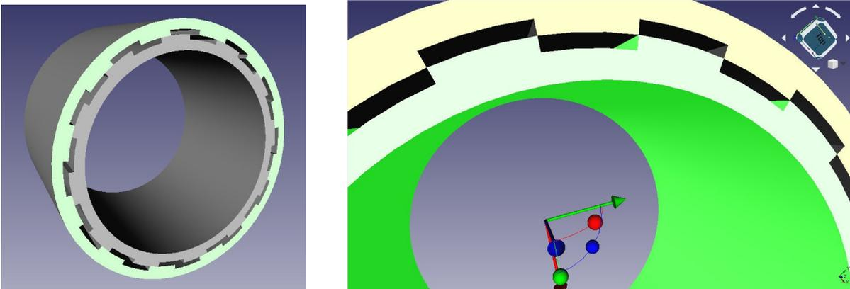
The device consists of an inner and an outer tube, each made of conducting material. The matching surfaces are splined so the capacitance between them varies as one or the other rotates. The splines run the length of the tubes, and the capacitances (as discussed in the Theory section) can be calculated as follows. It is assumed the splines and gaps are equal in angle.
